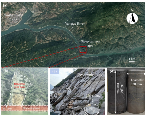
Note: (a) Wushan section of the Three Gorges Reservoir Area, (b) Fluctuation zone of steep banks, (c) Sampling location, (d) Fractured limestone specimens.
